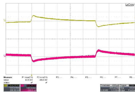
Transient Response to Dynamic Load Change from 100% to 75% of Full Load ; V_{in}=V_{in\ nom}
