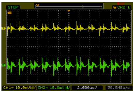
Typical Output Ripple and Noise V_{in}=V_{in\ nom} ; Full Load
