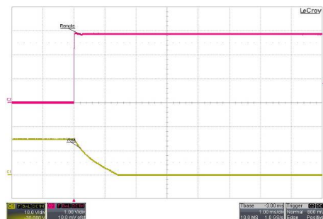
ON/OFF Voltage Start-Up and Output Rise Characteristic V_{in}=V_{in\ nom} ; Full Load
