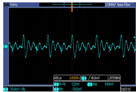
Typical Output Ripple and Noise V_{in}=V_{in\ nom} ; Full Load (-Vout)
