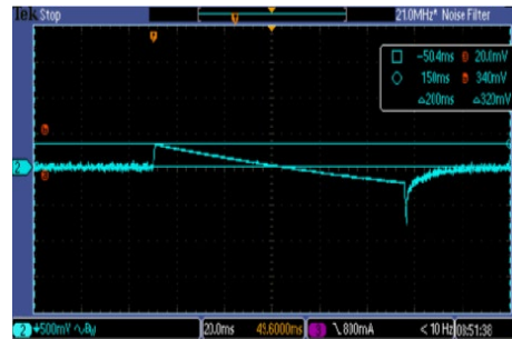
Transient Response to Dynamic Load Change from 100% to 75% of Full Load ; V_{in}=V_{in\ nom} (-Vout)
