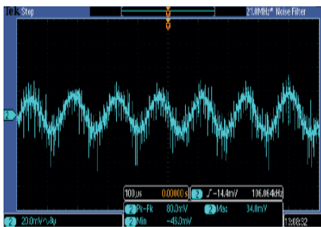
Typical Output Ripple and Noise V_{in}=V_{in\ nom} ; Full Load (+Vout)
