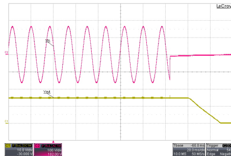
Typical Input Hold-up and Output Rise Characteristic V_{in}=V_{in\ nom} ; Full Load
